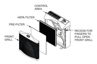
Fig. 2 - Air Purifier Components
